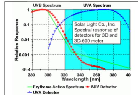
Fig. 1. Model 3D Spectral Response
