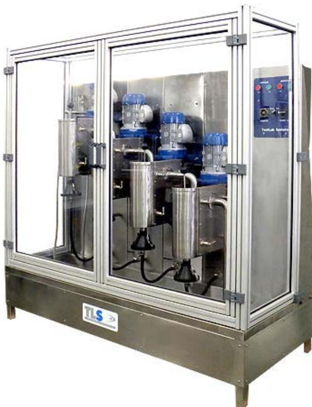
A green lamp shows that the agitation is in progress. During this time the drainage cups are furnished with weighed and marked filter papers. After the test (20 minutes according to TAPPI, 15 minutes according to SCAN) the stirrers will stop automatically and the green lamp of agitation goes out. Now shut off the water and as soon as the overflow from the last tank has nearly ceased, press the ON button of Vacuum for drainage after the completion of the agitation period.
