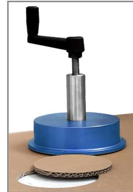
*\* Cutting ensured samples up to 10 mm thick*
