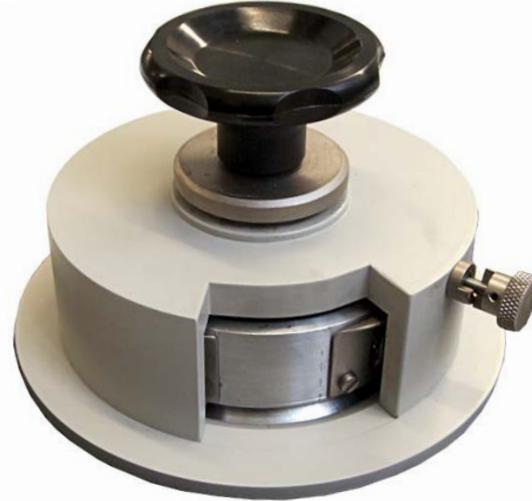
\* To cut Corrugated Board of a Thickness up to 7 mm maximum
