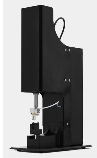
The Dia-Stron Interfacial Shear Strength module (IFSS) is an interchangeable module for the LEX820 high resolution extensometer used to measure the debonding force of micro-droplets on single filaments and fibres.
