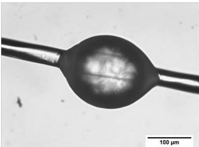
Above: Lyocell fiber with polypropylene droplet
