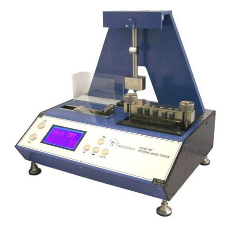
The new IBT Internal Bond Tester realizes a dynamic measuring principle to determine the internal bond strength of paper, board and compound materials. The significant influences of sample preparation and climatic conditions became consideration in the construction.
