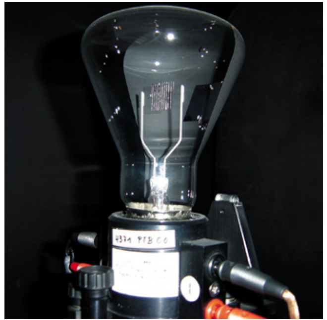
W141G standard intensity calibration bulb
