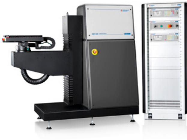
Goniophotometer used for luminous intensity measurement
