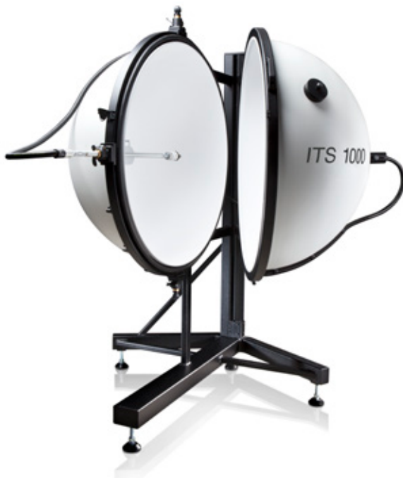
Integrating sphere for luminous flux measurement
